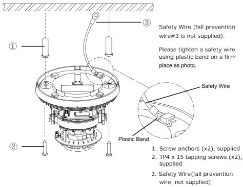
Figure 2-2 Camera installation
